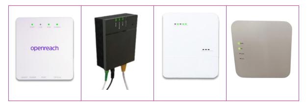
**Power light**: Check that the power light is green. Make sure the ONT is turned on at the mains, then check:
